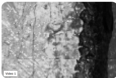
Figure 10: MA-XRF map for lead (Pb). Camille Pissarro, The Banks of the Oise near Pontoise , 1873, Indianapolis Museum of Art at Newfields, James E. Roberts Fund, 40.252.
